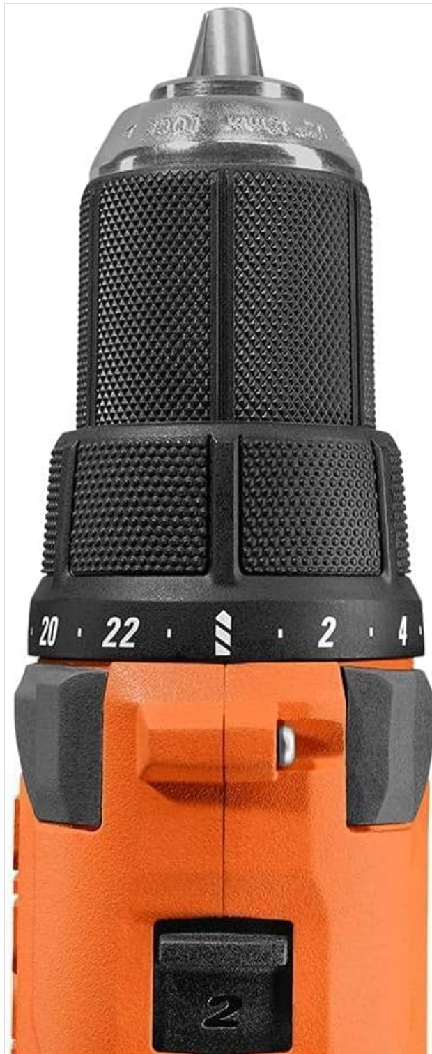
Figure 3.3: Top-down view of the chuck, clutch ring, and speed selector switch on the RIDGID R86001. The chuck is a 1/2 inch single sleeve ratcheting type, and the clutch ring has 24 positions for torque adjustment. The speed selector allows switching between two gear settings.
