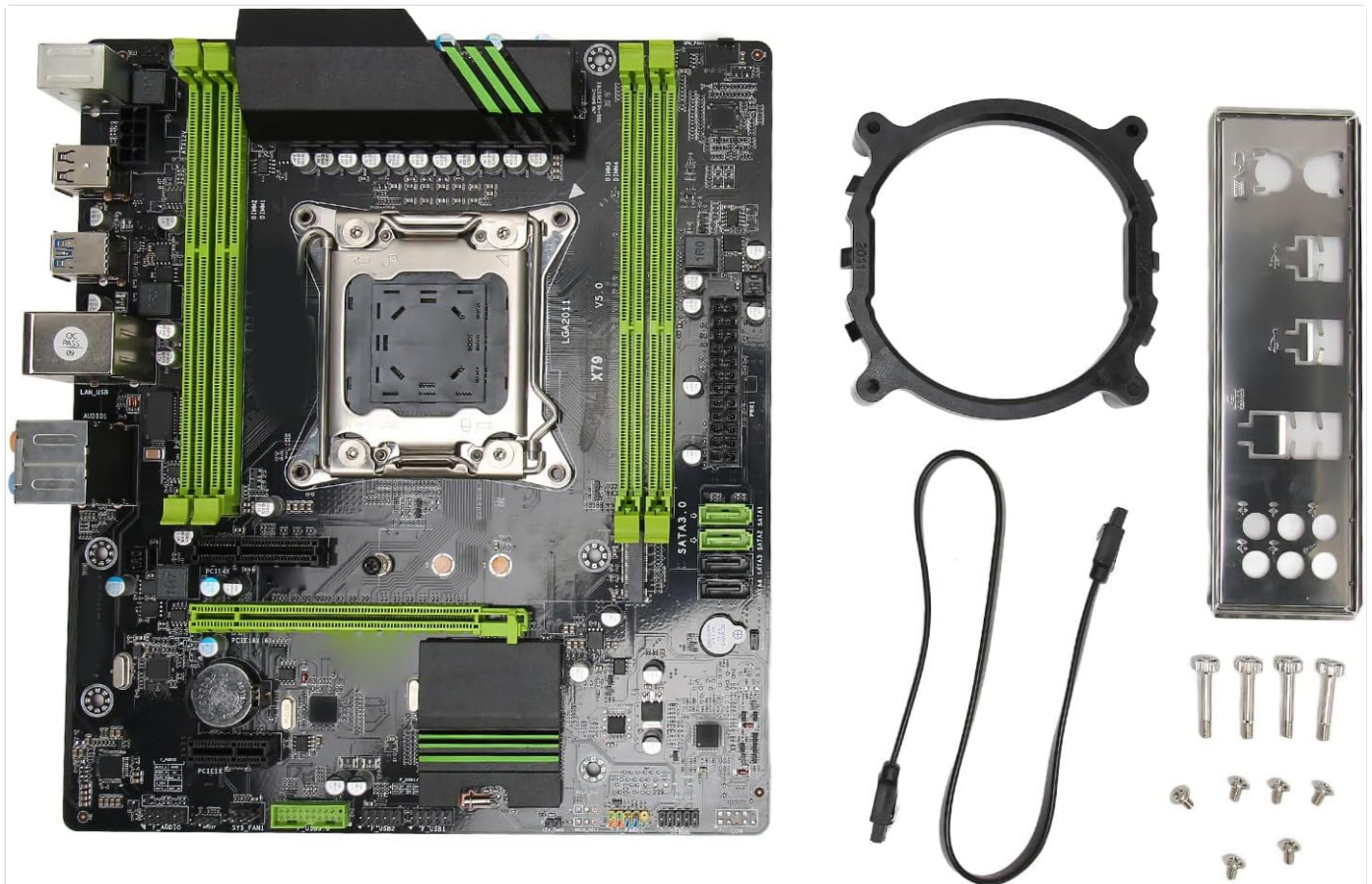
Image 3.1: Contents of the Bewinner X79 Motherboard package, including the motherboard, I/O shield, CPU cooler bracket, connection cable, and screws.
