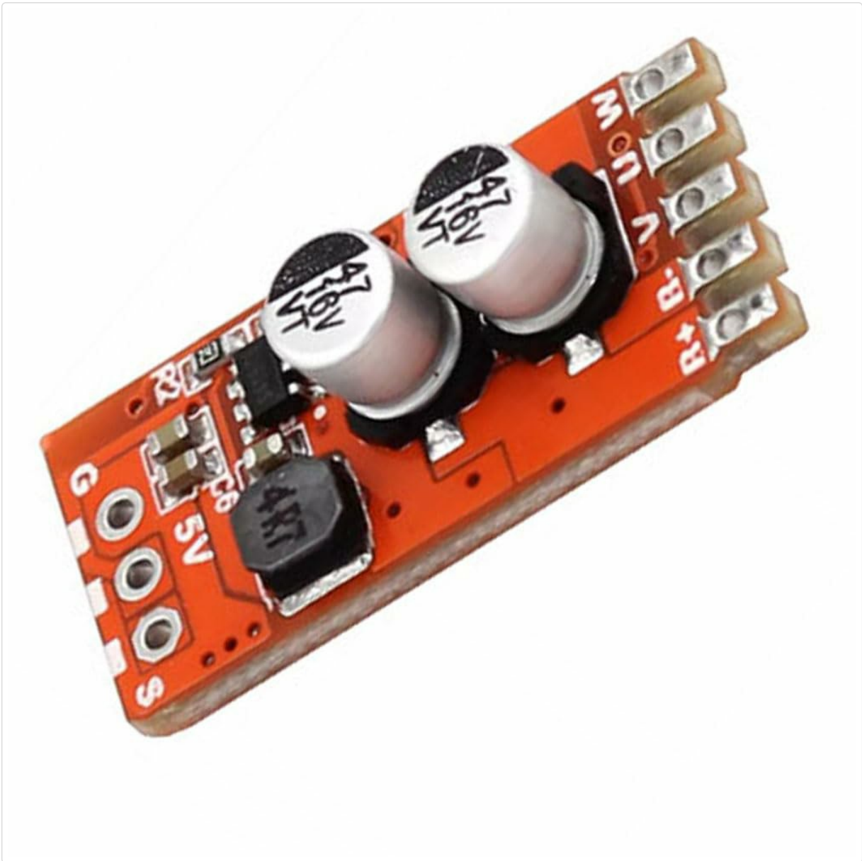
Figure 2: Angled view of the APO-C1 module, illustrating the power conditioning capacitors.
