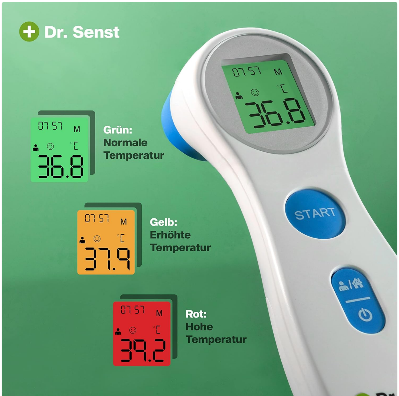
Image: The thermometer display showing examples of green (normal), yellow (elevated), and red (high) temperature readings with corresponding values.
