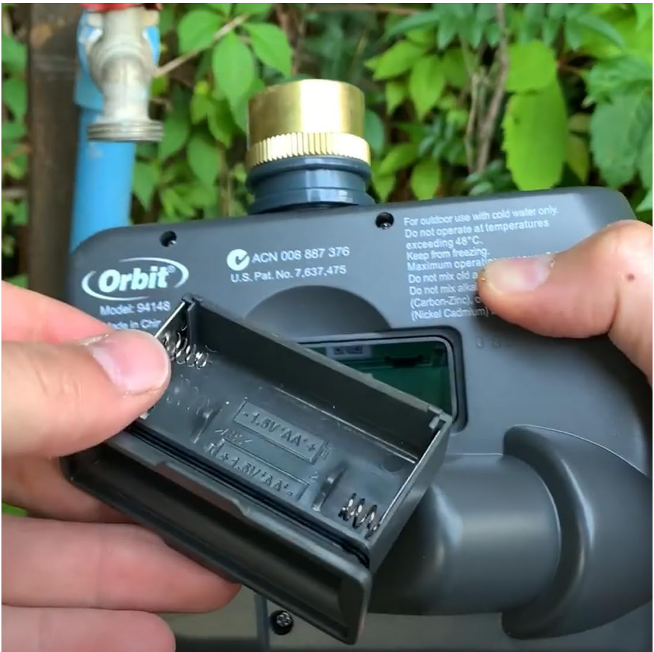
Image: A pair of hands demonstrating the opening of the battery compartment on the back of the GNCGarden Orbit Buddy II irrigation programmer. The compartment is designed for two AA batteries, and the image shows the springs and battery slots.
