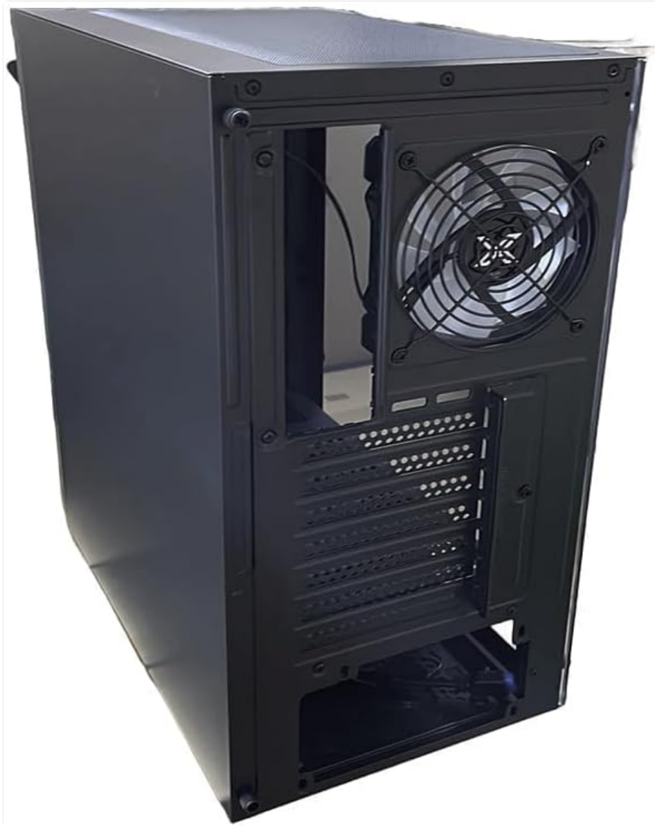
Figure 2: Rear view of the Xigmatek Blade ATX Computer Case, showing the power supply mounting area, expansion slots, and the exhaust fan.
