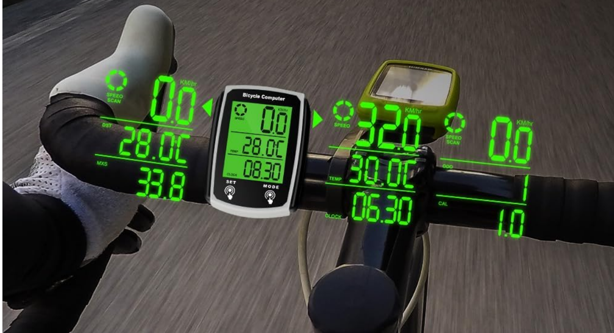
Image: The bicycle computer display showing real-time riding data, including speed, temperature, and clock, with multiple interface options.
