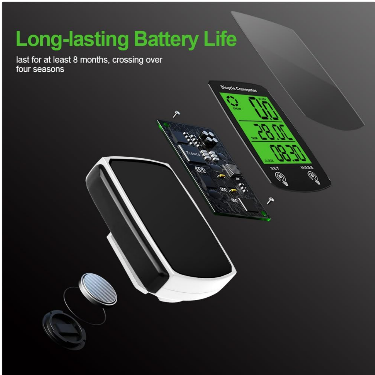
Image: An exploded diagram of the bicycle computer, illustrating its internal circuit board and the location of the coin cell battery, emphasizing its long-lasting battery life.
