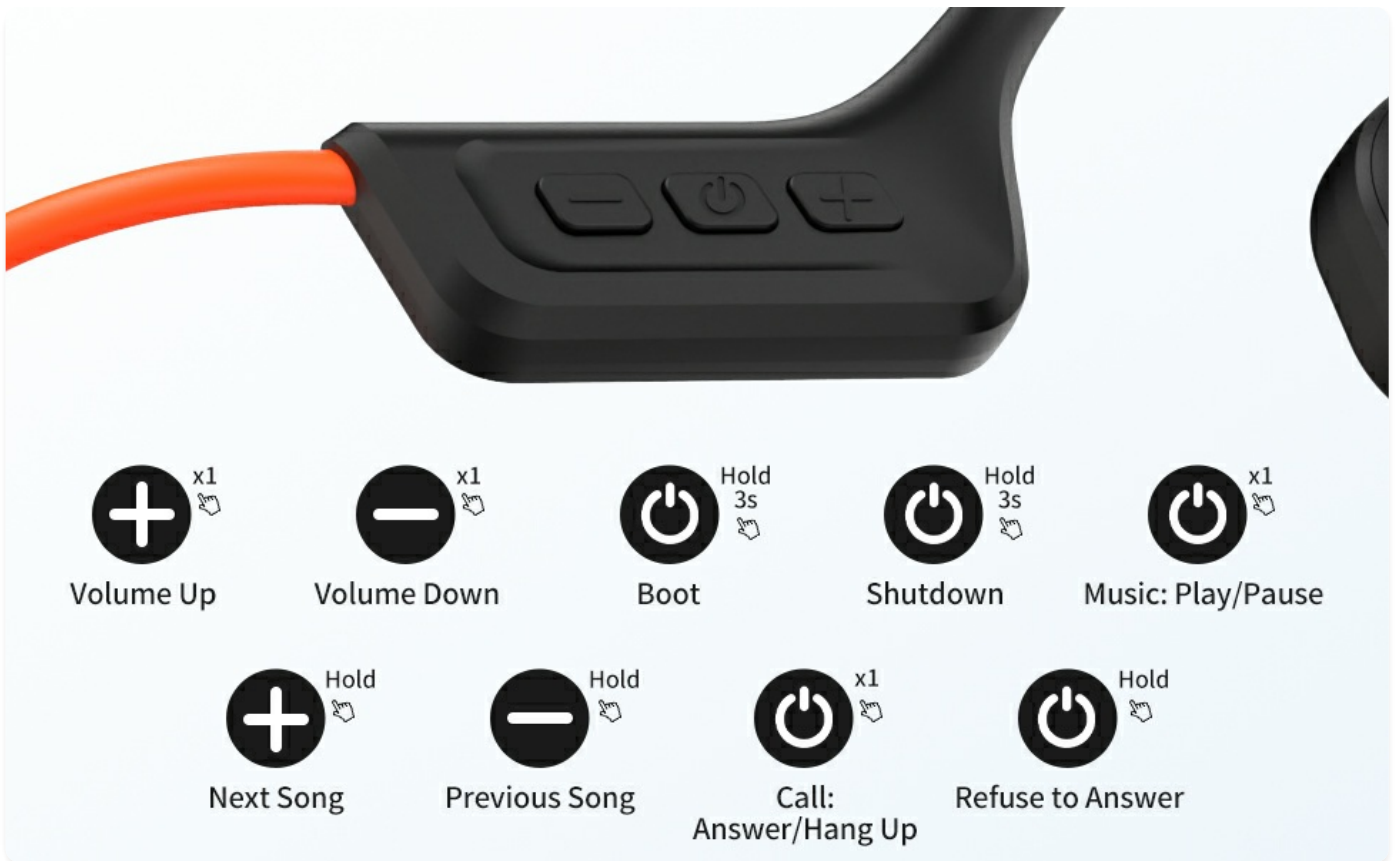
Image: A visual guide detailing the functions of each button for music playback and call management, including single clicks and long presses.
