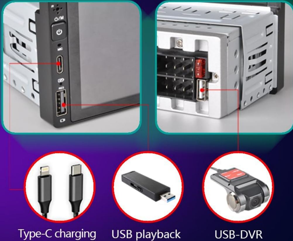
Figure 4.2: Illustration of the unit's connectivity options, including Type-C port for charging, front USB for media playback, and rear USB for DVR connection.
