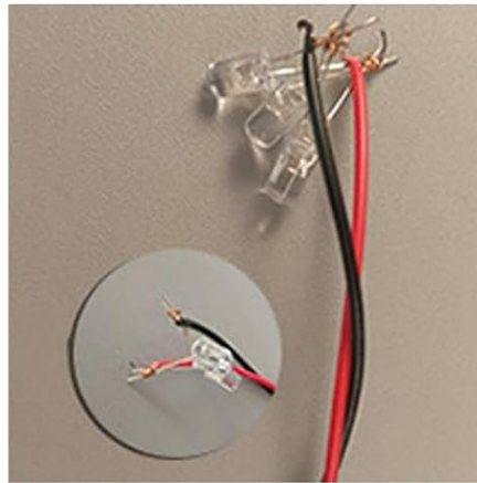
The LED light pins on both sides and the output copper wire cannot touch together to avoid short circuit
