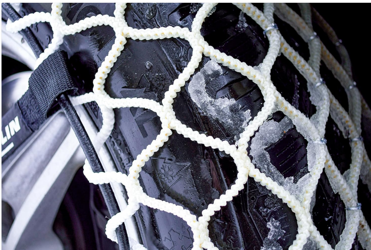
Image 4.2: A close-up view of the textile mesh and galvanized rings of the MICHELIN Easy Grip Limited snow chain, highlighting the material and construction that provide grip on ice and snow.
