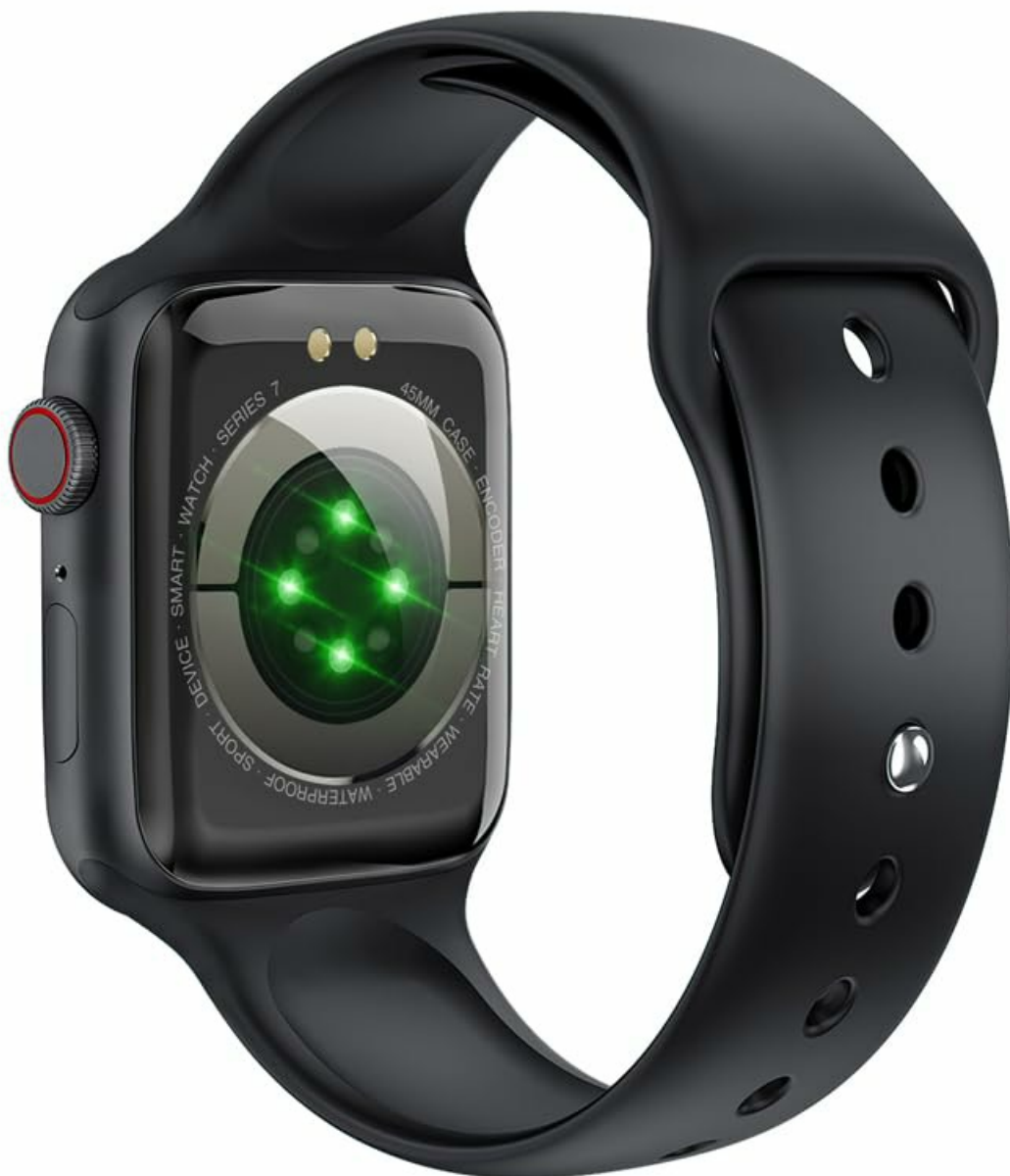
Figure 6: The rear view of the HOCO Smart Watch Y5, highlighting the optical heart rate sensors and charging contacts.
