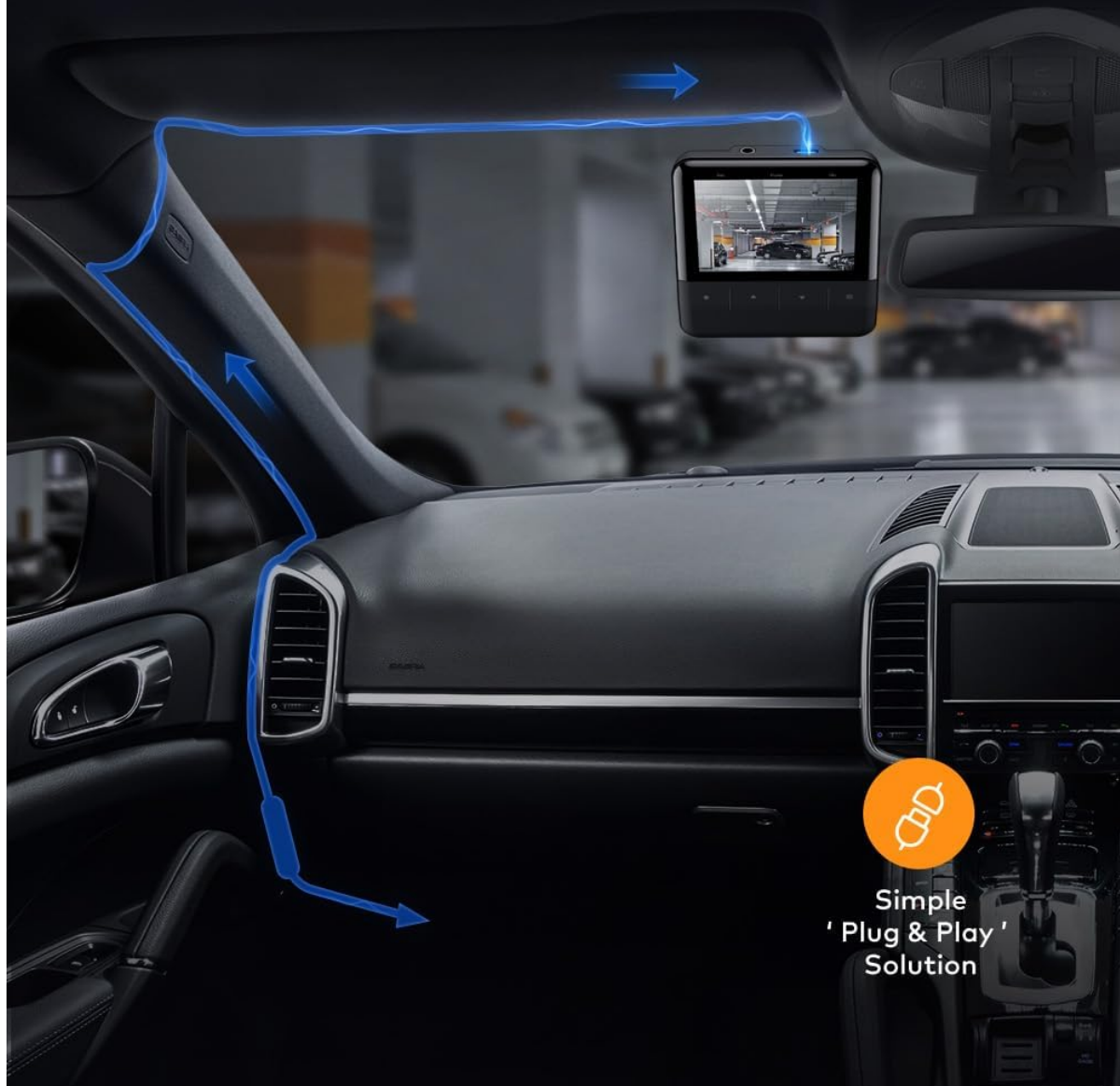
Image 3.1: Diagram illustrating discrete wiring of the hardwire kit from the OBD-II port to the dash cam.
