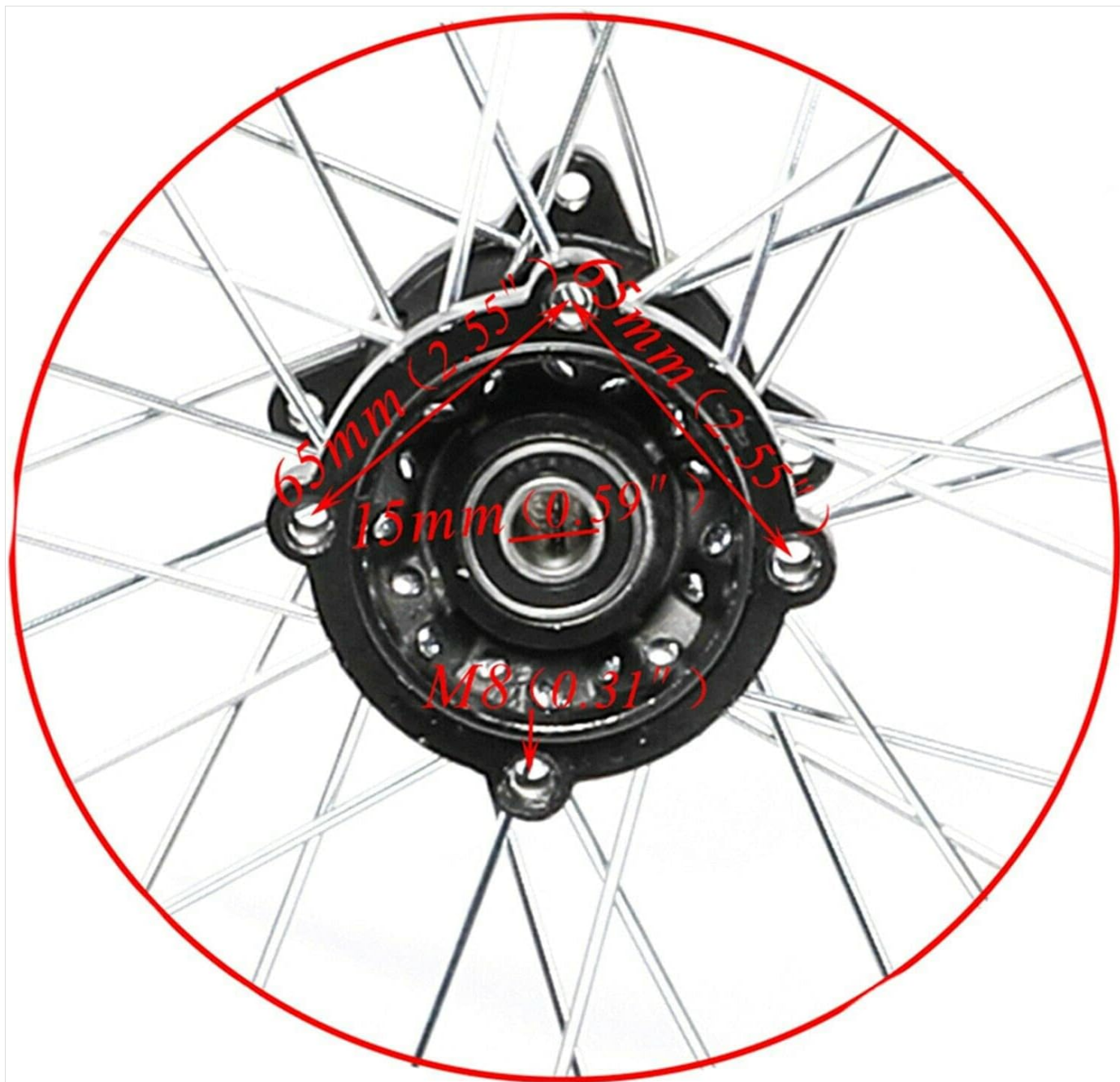
Figure 3: Close-up of the wheel hub, showing the 15mm axle hole and M8 tapped holes for mounting, along with pitch-row dimensions.
