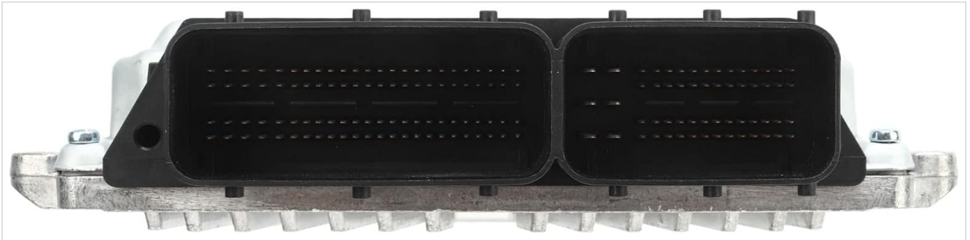
Image 3.1: Detail of the electrical connectors on the ECM, showing the pin configuration for connection to the vehicle's wiring harness.
