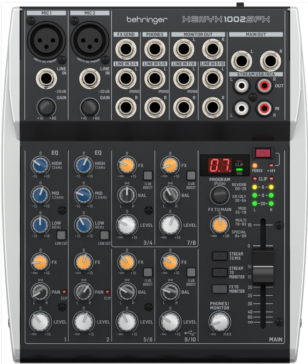
Figure 3.1: Front panel view of the Behringer Xenyx 1002SFX mixer, showing all inputs, outputs, and control knobs.
