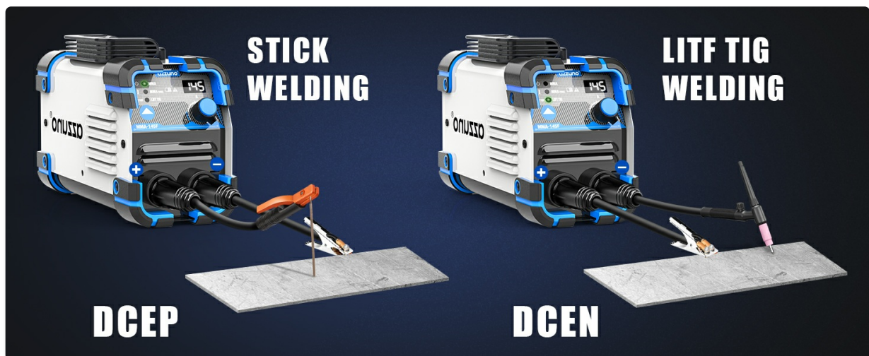
Image 4.2: Visual guide for connecting welding cables, illustrating Direct Current Electrode Positive (DCEP) for Stick welding and Direct Current Electrode Negative (DCEN) for Lift TIG welding.
