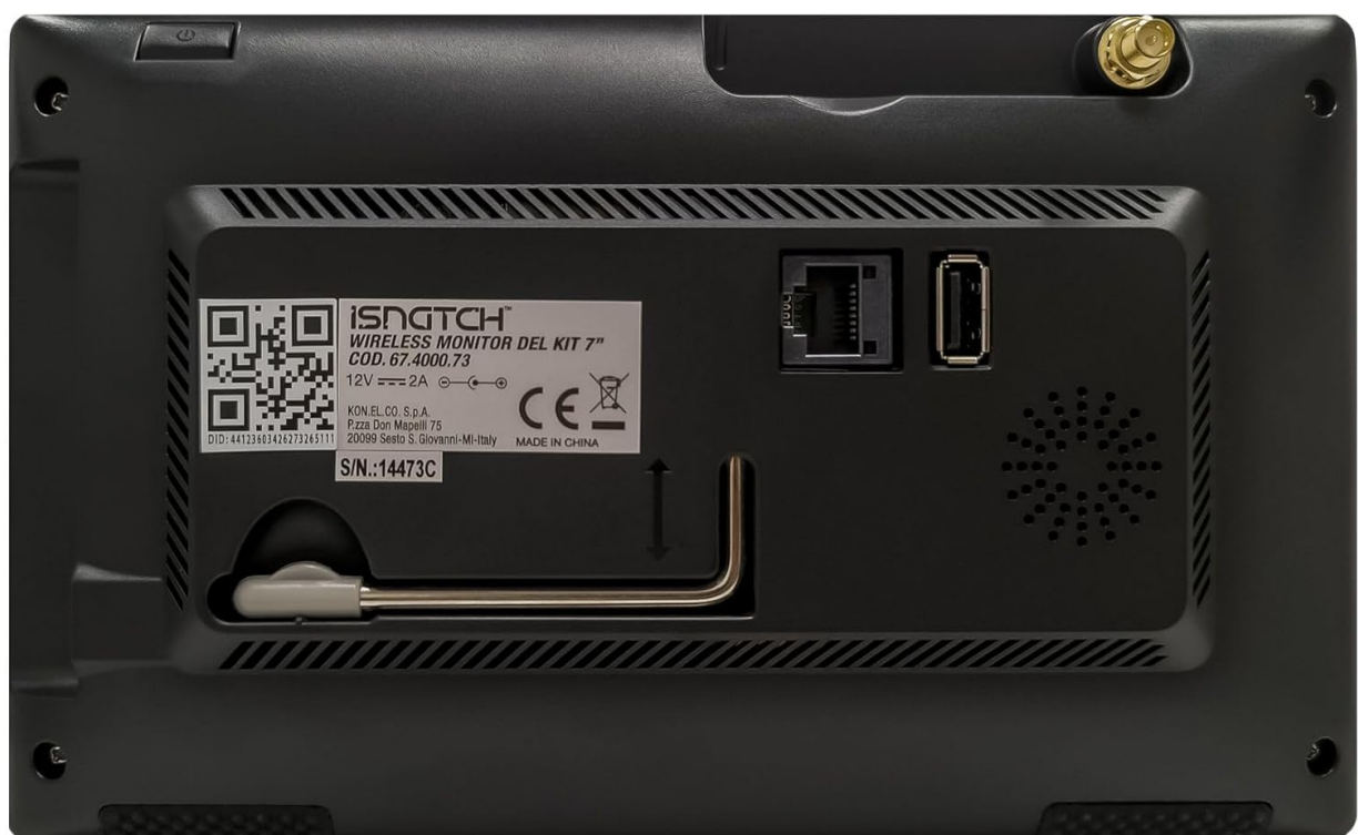
Figure 4.2: The rear panel of the ISNATCH monitor, displaying the LAN port, USB port, power input, and a QR code for product information. The QR code links to 44123603426273265111 .
