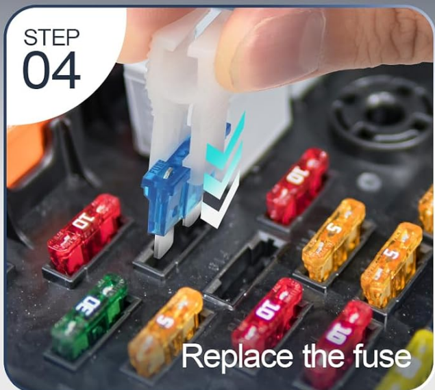
Figure 2.1: Step-by-step visual instructions for replacing a vehicle fuse.
