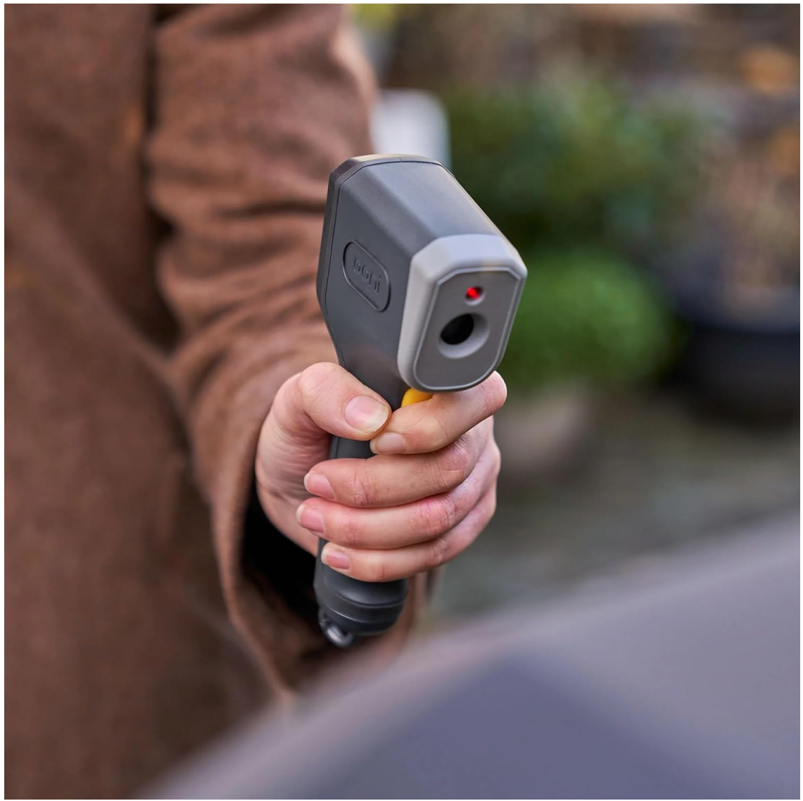
Figure 4: A hand holding the Ooni thermometer, with the red laser dot visible, indicating the measurement target.
