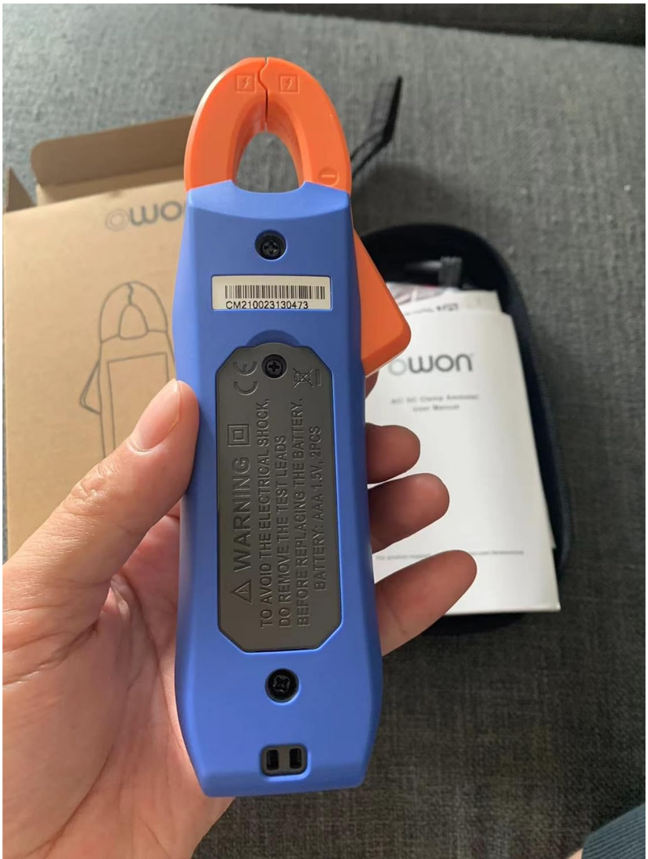
Image: The rear of the CM2100B meter, displaying the battery compartment cover and a warning label regarding battery replacement.
