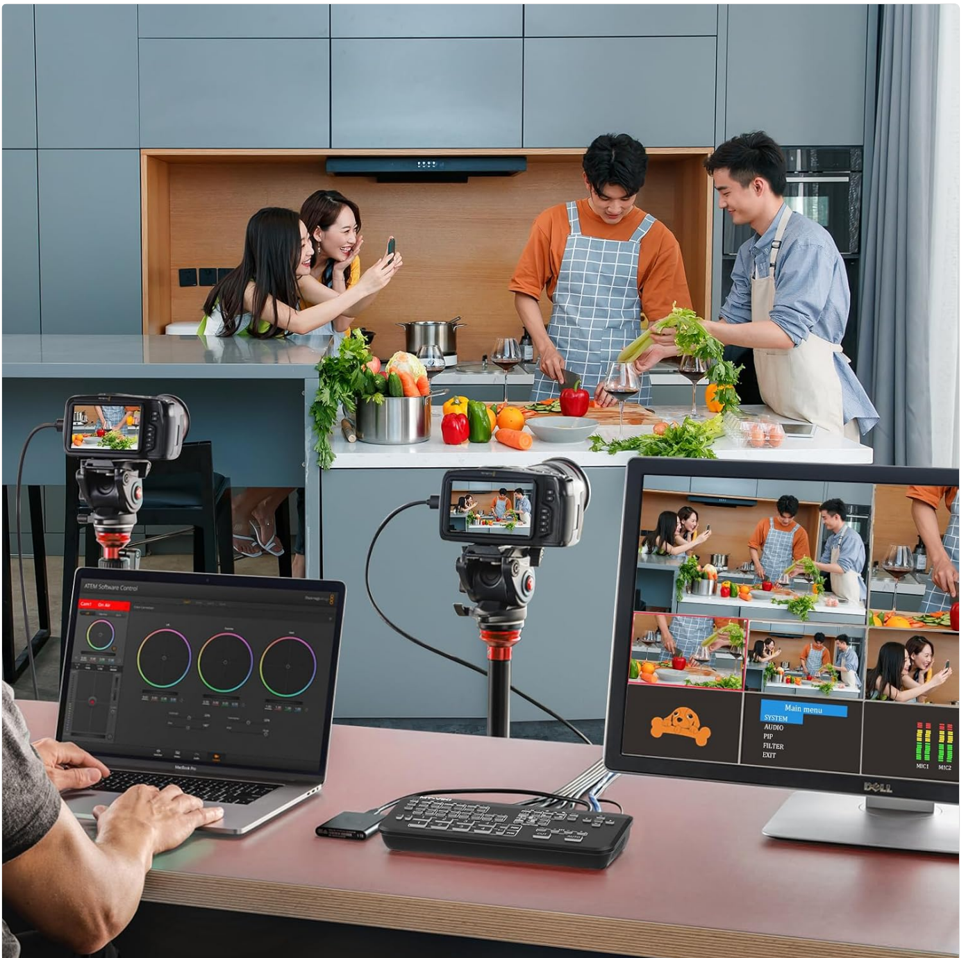
Image 5.1: Example Setup. This image illustrates a typical setup with the MT-VIKI switcher connected to multiple cameras, laptops, and external monitors, demonstrating a multi-source live production environment.
