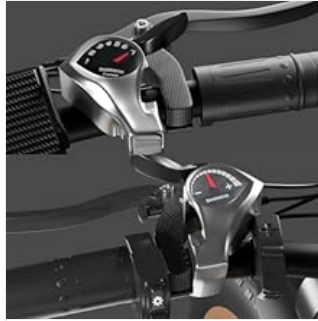
Image: Close-up of the Shimano gear shifters on the handlebar, indicating the current gear selection.
