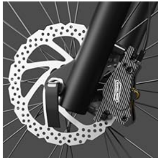
Image: A detailed view of the front hydraulic disc brake system, showing the caliper gripping the rotor.
