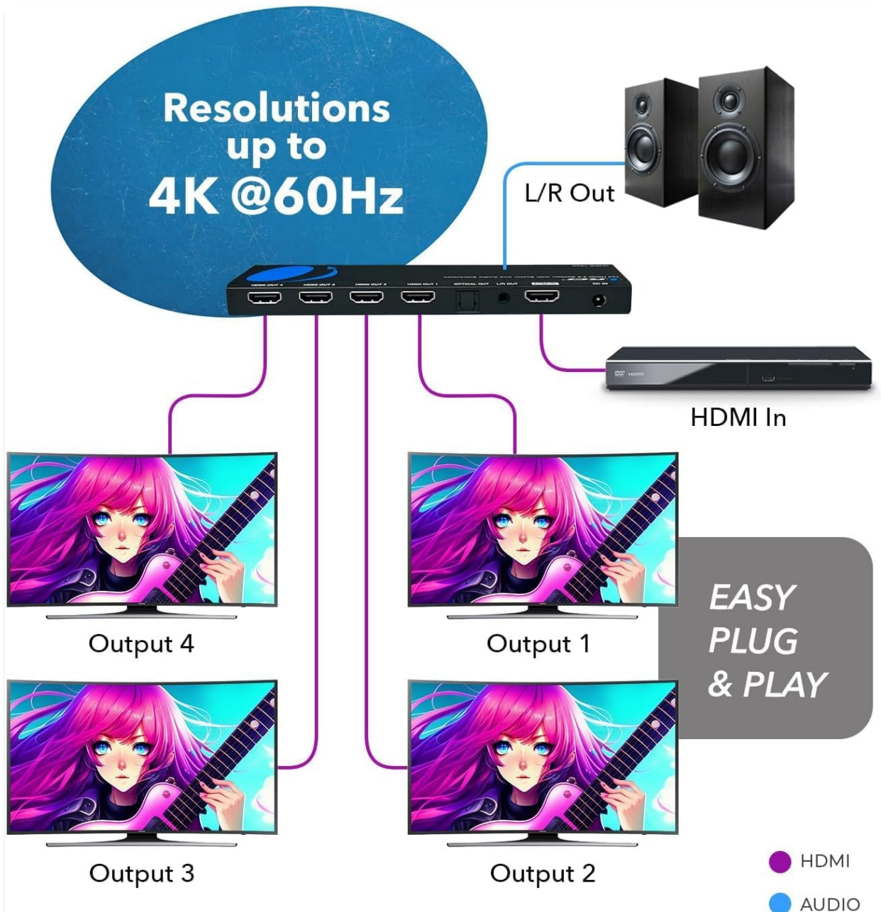
Figure 5: Diagram illustrating the typical connection setup for the OREI UHDS-104A, showing source, splitter, displays, and audio output.
