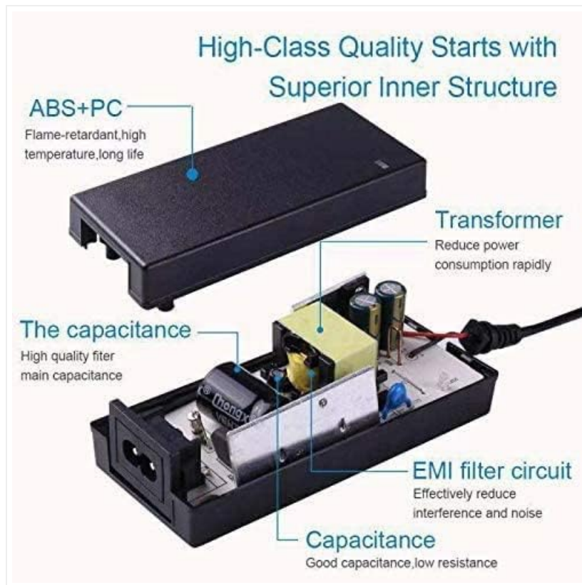
Figure 4: Exploded view showing the internal components of the charger, including the transformer, capacitance, and EMI filter circuit, designed for stable output and reduced interference.
