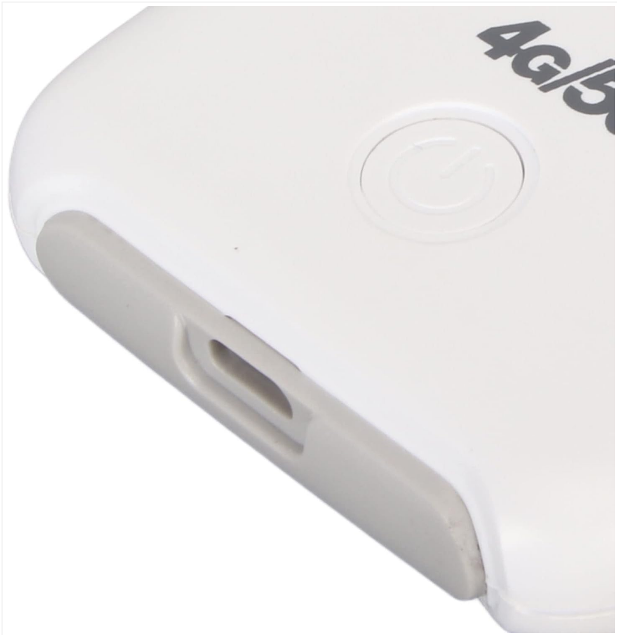
Figure 3.3: Micro USB port.
