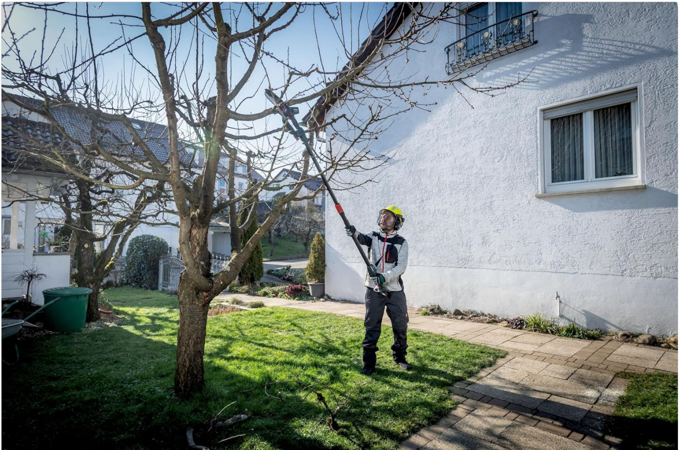
Figure 9: Extending reach with the optional telescopic handle for high pruning tasks.
