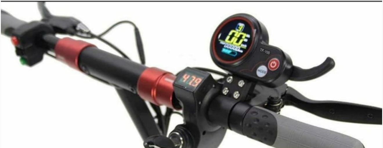
Image: The TF-100 throttle unit, highlighting its 6-pin connector and indicating compatibility with 36V-48V systems.
