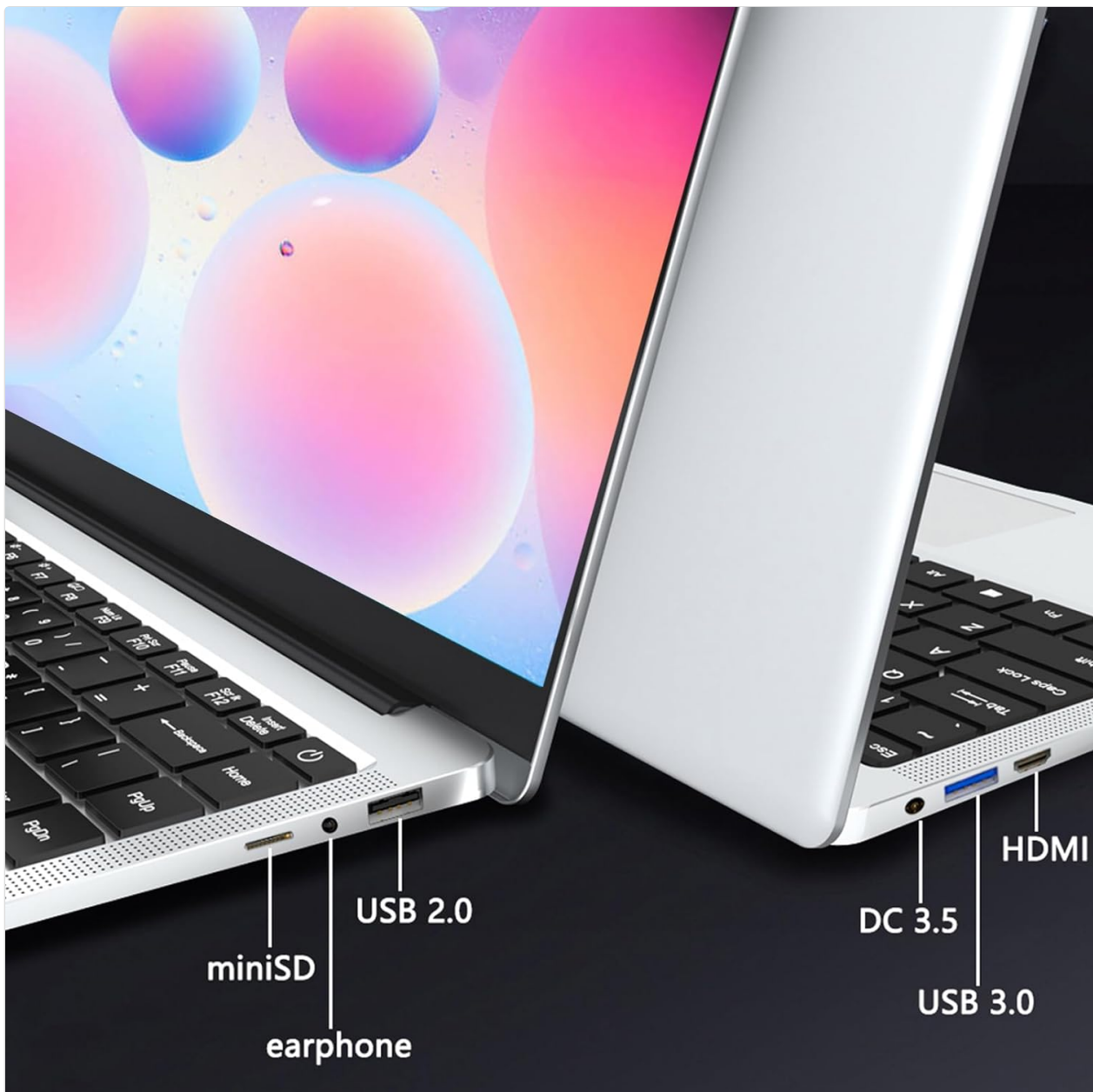
Figure 4.4: Side view of the KUU XBOOK-3 Laptop, highlighting the available ports for connectivity, including miniSD, earphone jack, USB 2.0, USB 3.0, DC 3.5 charging port, and Mini HDMI.
