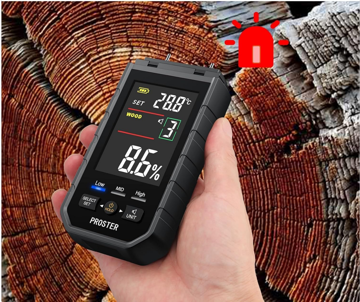
Figure 4.4: The meter displaying a high moisture reading with an high moisture level indicated by a red alarm icon.
