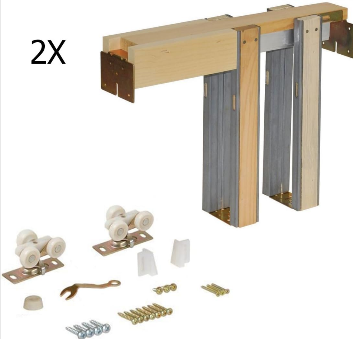
Figure 3: All components included in the SARTODOORS double pocket door kit. This image displays the pocket frames, track, hangers, door guides, bumpers, pulls, and mounting screws.
