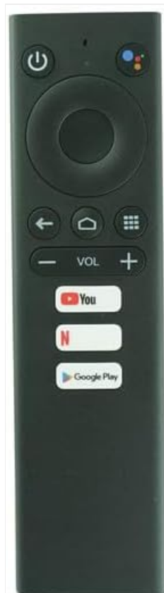
Figure 1: Front view of the remote control, showing the power button, Google Assistant button, circular navigation pad, back, home, menu,
