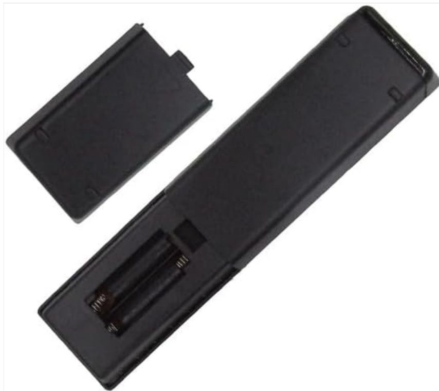
Figure 3: Rear view of the remote control with the battery cover detached, revealing the compartment for two AAA batteries.
