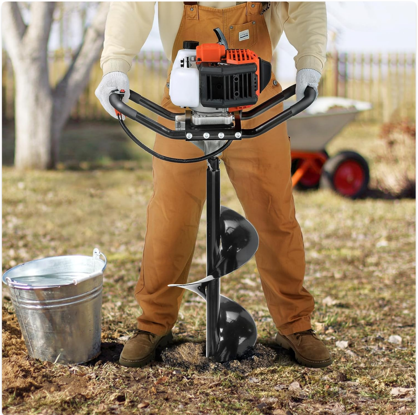
Figure 4: Proper operating stance for the VEVOR Post Hole Digger.
