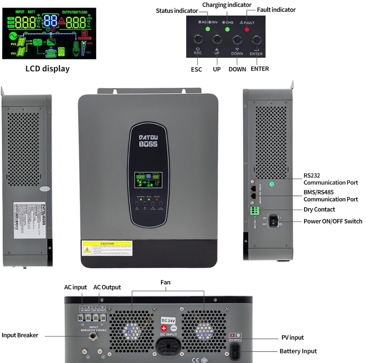
Figure 2: Inverter Front, Side, and Rear Views with Labels
