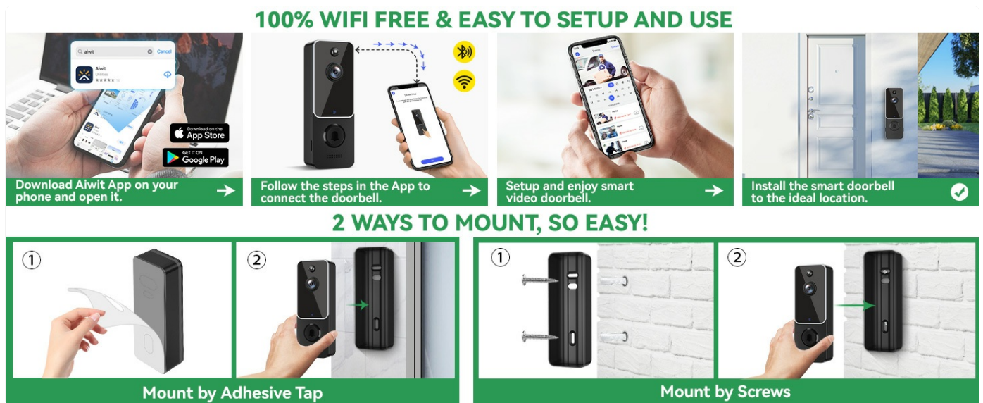
Image: Step-by-step guide for app setup and physical installation using adhesive or screws.
