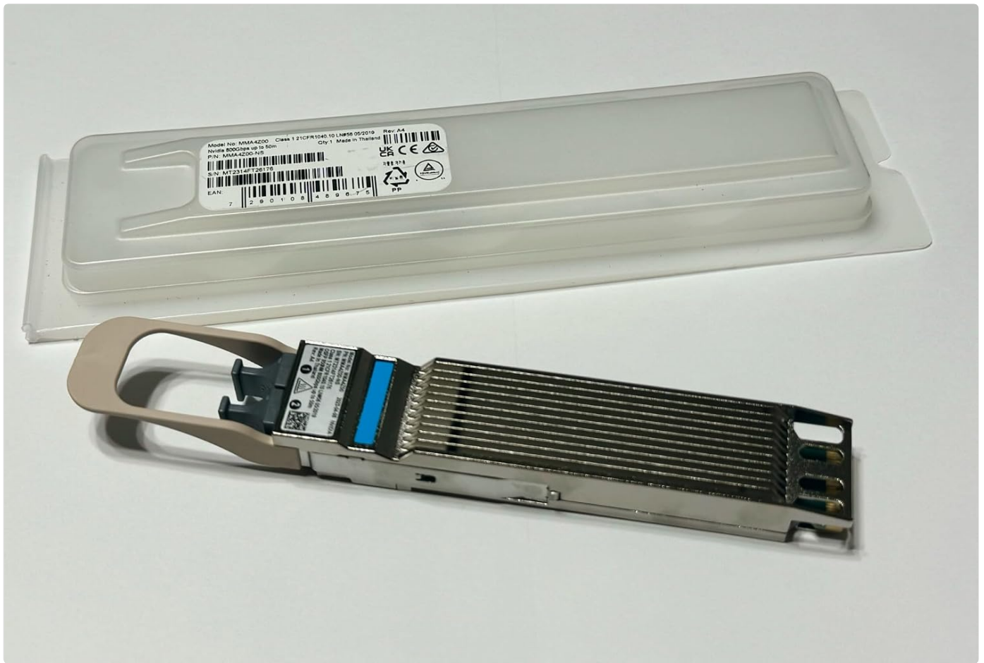
Figure 1: The NVIDIA MMA4Z00-NS OSFP transceiver shown alongside its clear plastic protective packaging. The transceiver features a metallic body with cooling fins and a beige pull tab. The packaging displays product information including model number MMA4Z00-NS and EAN 7290108489675.
