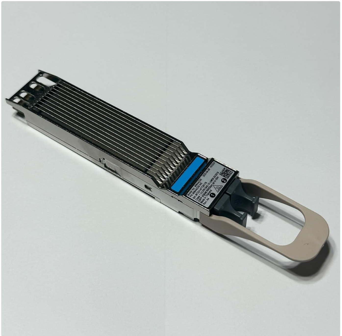
Figure 2: A detailed view of the NVIDIA MMA4Z00-NS OSFP transceiver, highlighting its metallic finned top for heat dissipation and the blue optical interface. This view emphasizes the robust construction designed for high-performance networking environments.
