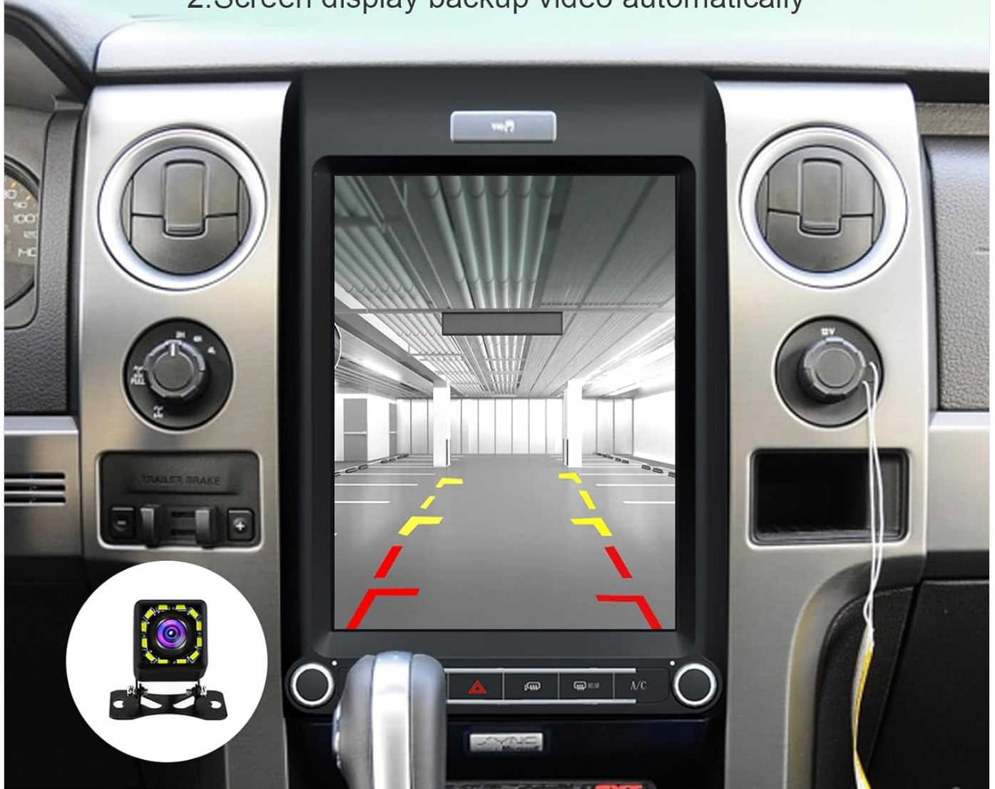
Figure 5: Automatic display of reversing video input with parking guidelines.
