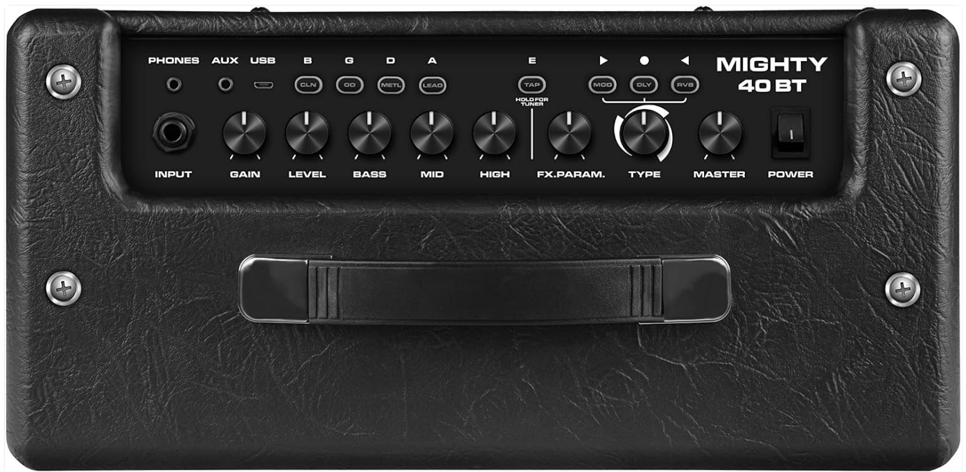
Image: Top panel of the NUX Mighty 40 BT amplifier, displaying various knobs and jacks for input, gain, level, bass, mid, high, FX parameters, type, master volume, and power switch.
