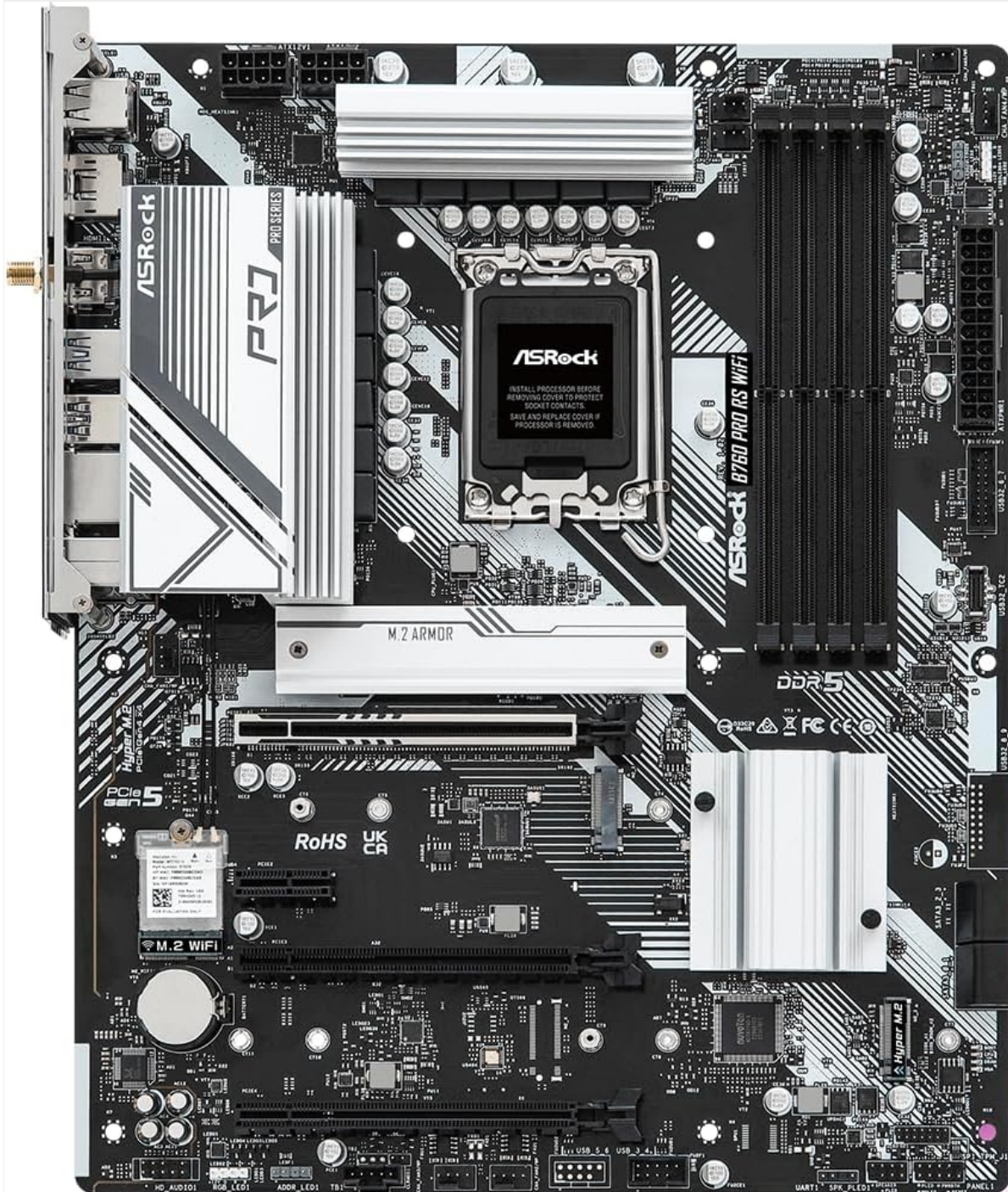
Figure 1: Top view of the ASRock B760 Pro RS WiFi 6E motherboard, showcasing the CPU socket, DIMM slots, PCIe slots, and heatsinks.
