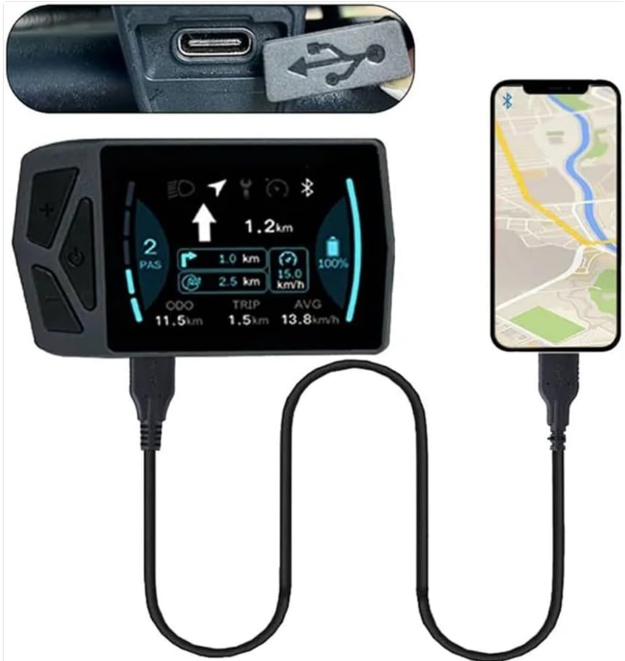
Figure 7.1: The RANRAO B02N display connected via USB-C to a smartphone, demonstrating its capability to display navigation information from a paired mobile application.
