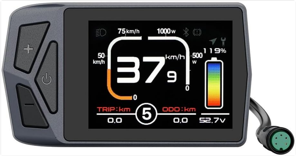
Figure 4.1: Front view of the RANRAO B02N Color LCD Display, showing the screen and control buttons (+, Power, -).
