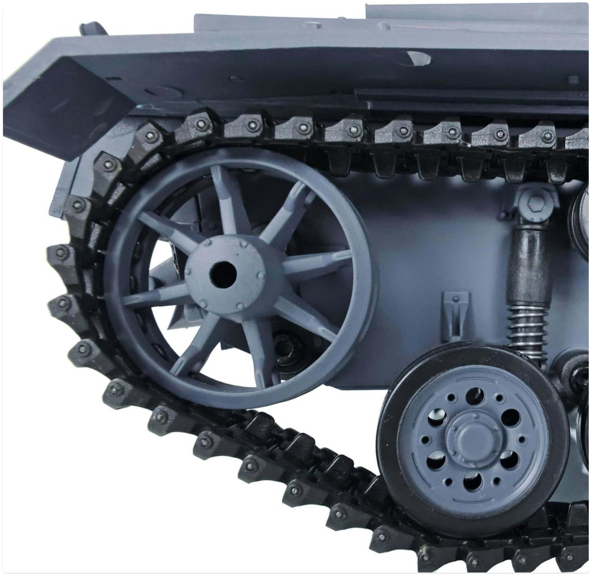
Image 5.1: Close-up of the tank's tracks and metal roadwheel suspension, important for maintenance checks.
