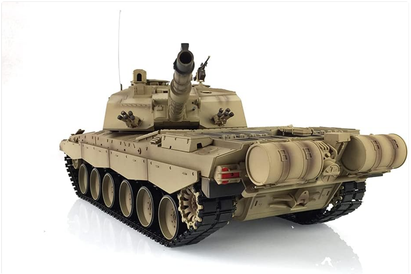
Figure 3: Rear view of the tank, showing the exhaust and external fuel drums.
