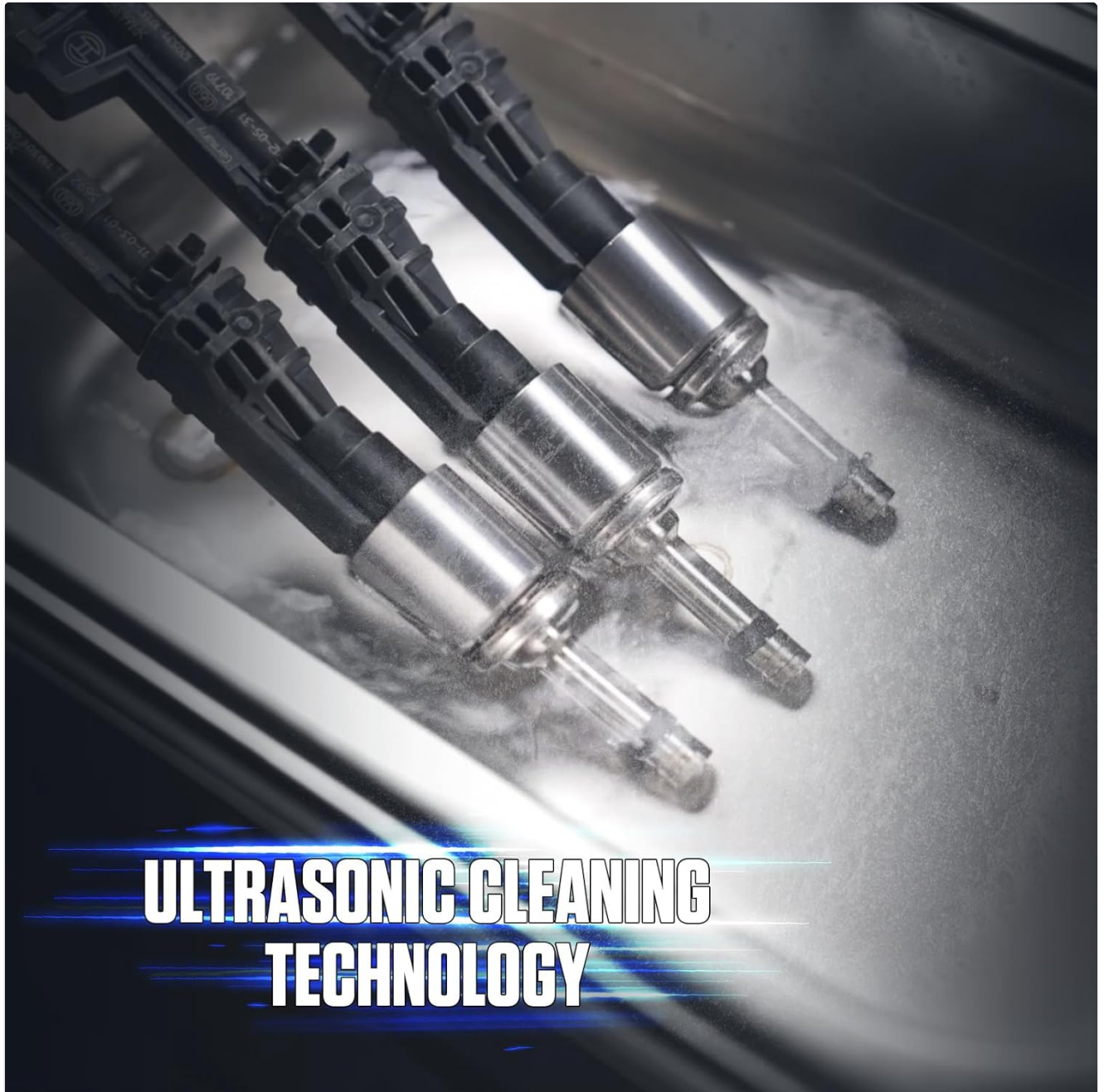
Image: Fuel injectors submerged in the ultrasonic cleaning tank, demonstrating the ultrasonic cleaning technology in action.
