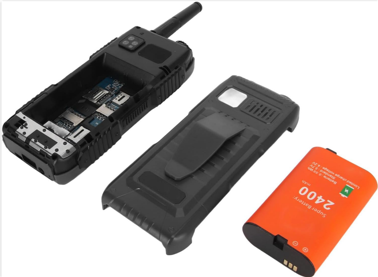
Image 3.1: Internal view of the phone with the back cover removed, showing slots for SIM cards and memory card.
