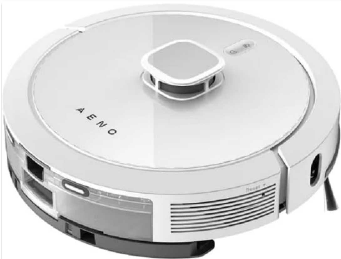
Figure 2.3: A side-top view of the AENO ARC0004S Robot Vacuum Cleaner, highlighting the removable dustbin and water tank compartment. This area is crucial for both dry vacuuming and wet mopping functions.
