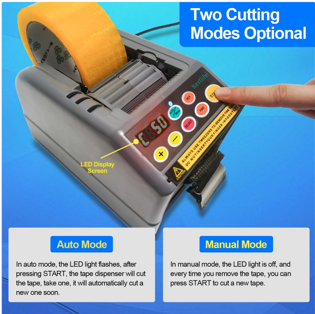
Figure 4: Control panel illustrating the two cutting modes.
