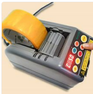
Figure 6: Pressing the START button to begin cutting.
