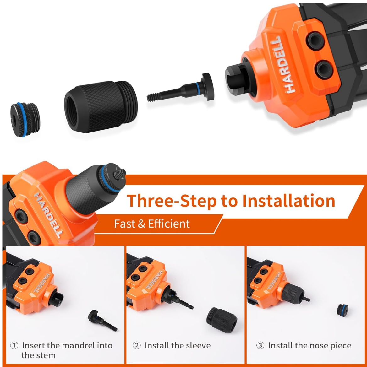
Image 3.1: Three-step mandrel installation process.
