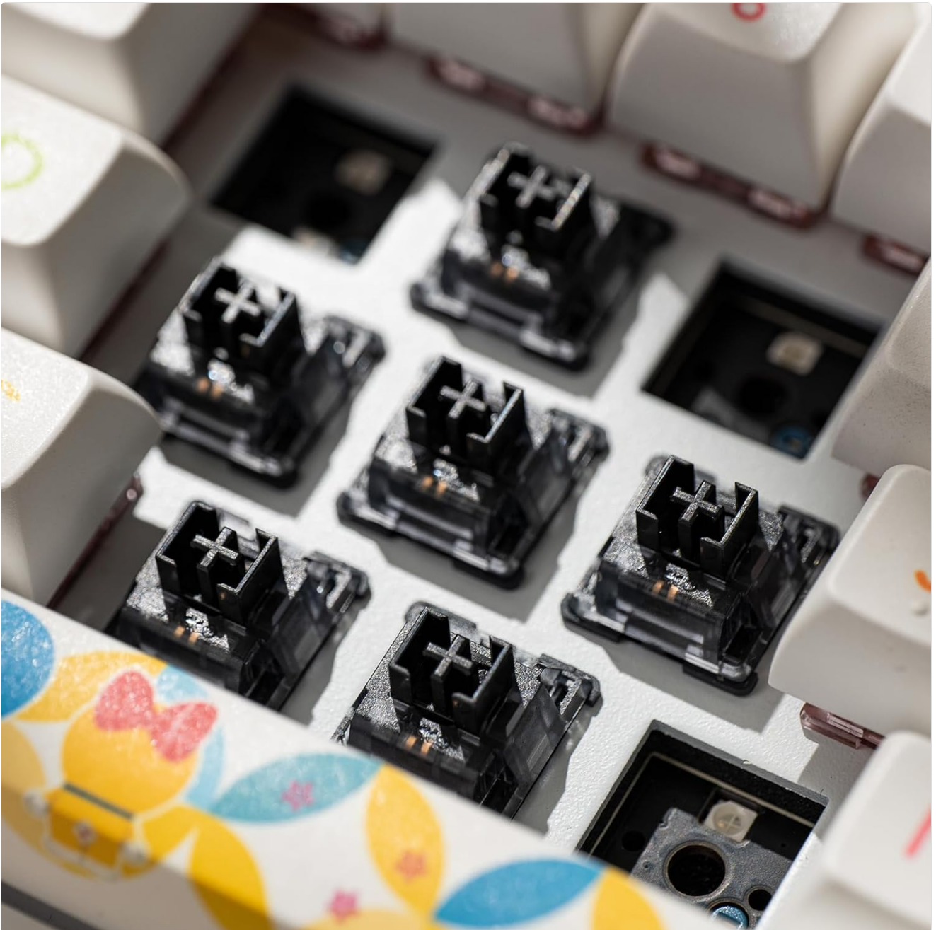
Image: Akko V3 Creamy Black Pro switches installed in a mechanical keyboard, showcasing their appearance.
