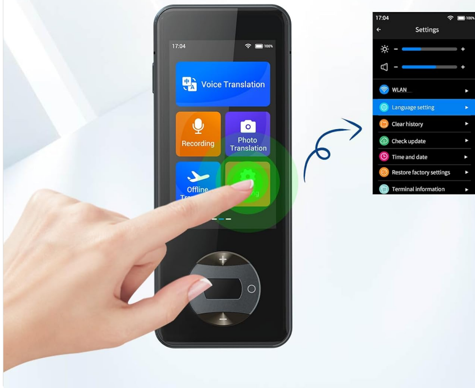
Figure 2: The device's 3.0-inch TFT(IPS) HD touch-screen, showing the main menu with options like Voice Translation, Sound Recording, Photo Translation, Offline Translation, and Settings.
