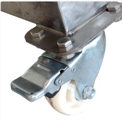
Figure 5: Close-up of a caster wheel with a locking mechanism, providing mobility and stability for the conveyor unit.
