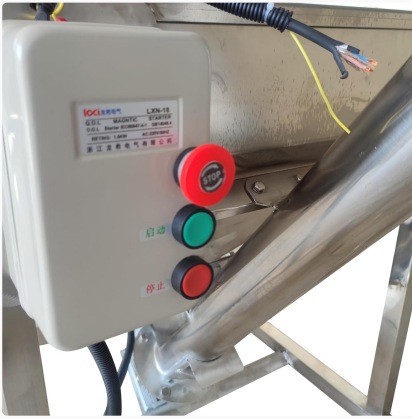
Figure 3: Close-up view of the control panel, featuring start (green), stop (red), and emergency stop buttons. The panel is clearly labeled for intuitive operation.
